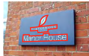
For a wall sign that is a panel mounted on the wall, the panel itself is the sign structure, and so is not considered to be a setting, and is not included in the sign message area.
