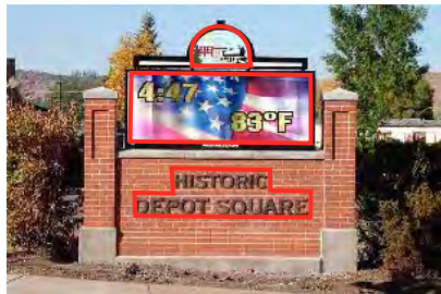
The graphic at the top of the sign, all of the LED screen, and the text are included in the sign message area.
